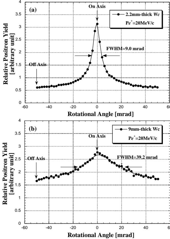
Figure 3: Relative positron yields (a) for the 2.2mm-thick  $W_c$  and (b) for the 9mm-thick  $W_c$  as a function of the goniometer rotational angle around the  $H$  axis while the angle around the  $V$  axis is fixed to the position giving the yield peak. The solid curves are only for the eye's guide.
