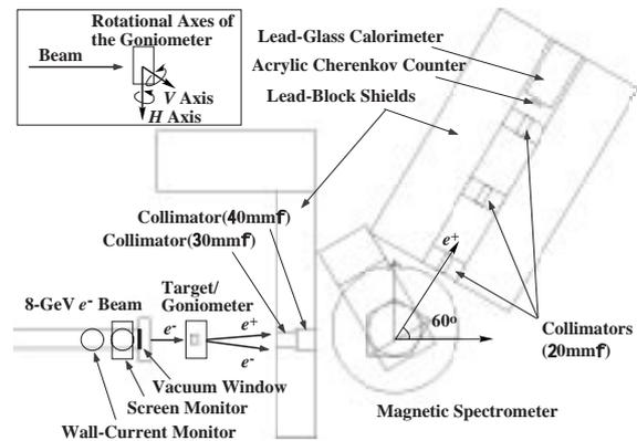
Figure 2: Schematic drawing of the experimental setup.
