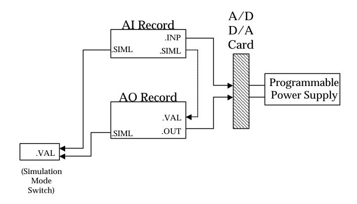
When in simulation mode, the AO record does not call device support and the AI record fetches its input from the AO record.
