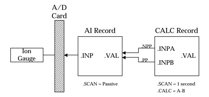
INPA fetches data that is 1 second old because it does not request processing of the AI record. INPB fetches current data because it requests the AI record to process. The subtraction of these two values reflects the 'rate of change' (difference/sec) of the pressure reading.
