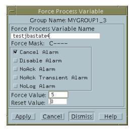
There are four action buttons on this dialog box: Apply, Cancel, Dismiss, and Help. The Apply button will accept and apply the user entered changes. The Cancel button will discard the user entered changes in this dialog box and reset them to the original values. The Dismiss button will close this popup dialog, and the Help button will display a Force PV help information dialog.
