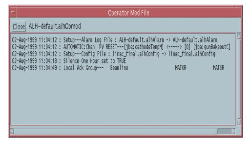
ALH does not allow an operator to view a log file that exceeds 1 Megabyte. When the log file exceeds 1 Megabyte, a new log file must be used in order for an operator to be able to
