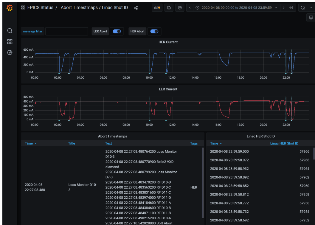
FIGURE 7.12: Abort Trigger System log displayed in Grafana.
