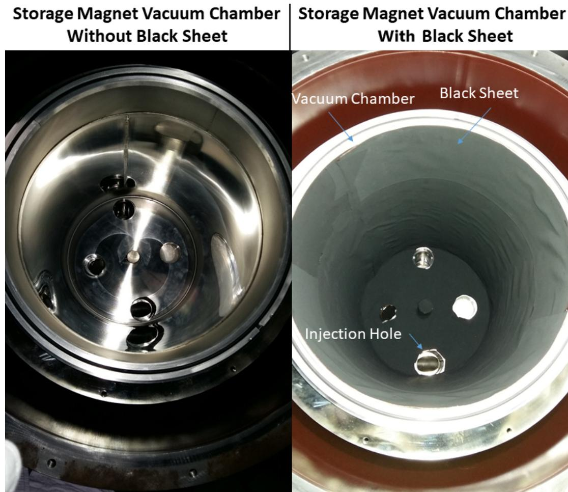
Figure 4.7: Left: Vacuum chamber without the black sheet. The light reflection from the wall of the vacuum chamber can be seen very clearly. Right: Vacuum chamber with the black sheet. The light reflection suppressed considerably after the insertion of the black sheet.
