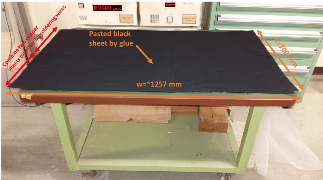
Figure 4.5: Two copper sheets of height (350 mm) had been joined together to make a copper sheet of height 700 mm. The black sheet of height 700 mm and width 1257 mm was attached to the thin copper sheet by Araldite Rapid Epoxy.
