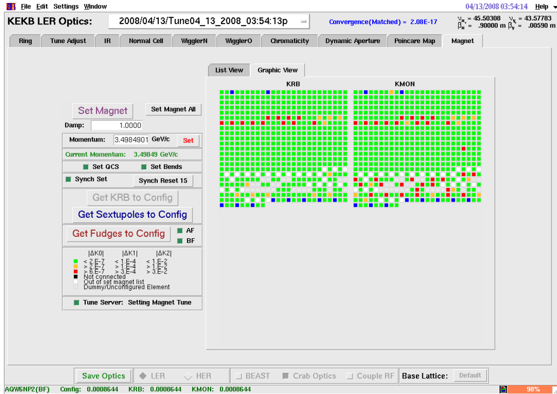
Figure 22: optics panel for the storage rings
