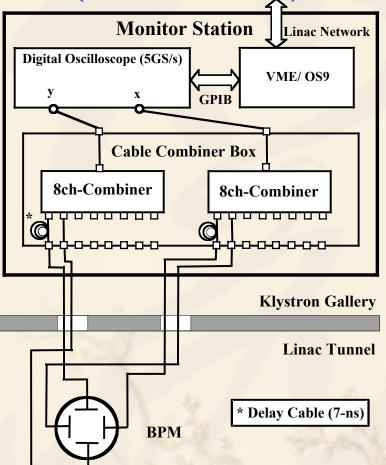
✓VME + Oscilloscope (TectronixTDS680, 5-GSa/s, 8-bits)
