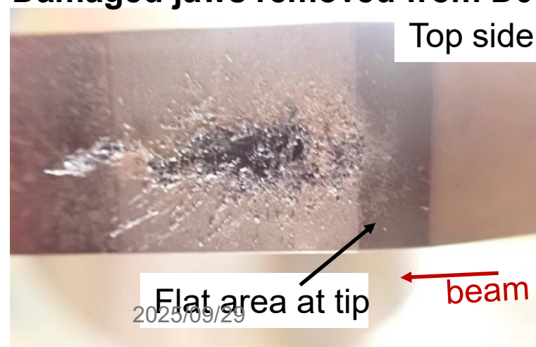
Damaged jaws removed from D05V1 (Ta, 4 mm)
