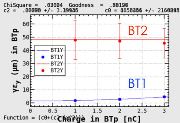
1. Since the horizontal emittance blowup seems to depend on the amount of charge, we suspected the influence of CSR and decided to move the e+ beam closer to the chamber inner wall of the first arc bend (BH1P) to see if the blowup would be reduced.
