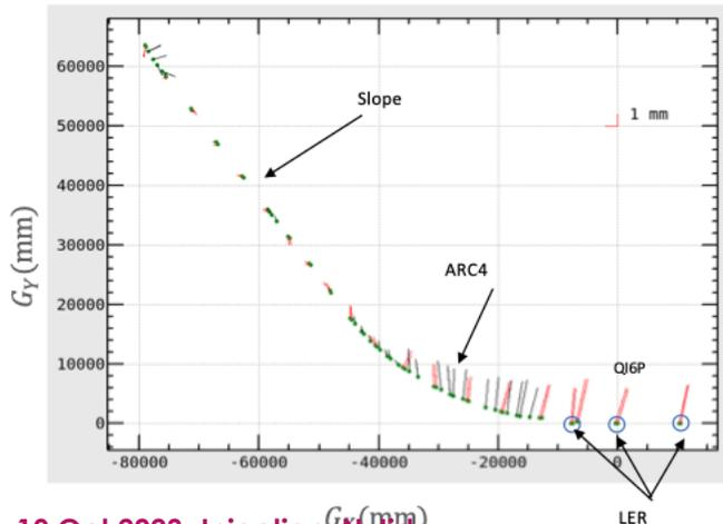
Analysis of measured electromagnet positions (2018)
