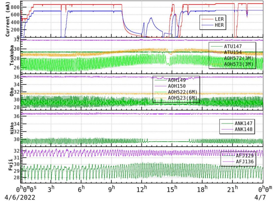
Temperature of vacuum cooling system is very stable.
