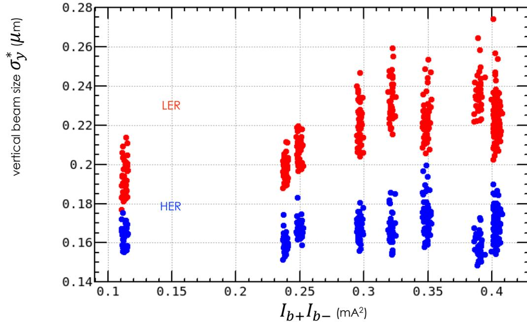
Beam size blowup is significant in LER.
