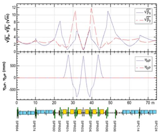
New optics at J-ARC with pulsed quads
