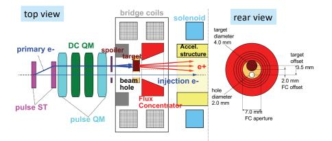
Figure 11.90: Target, FC offset layout
