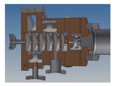
Figure 11.62: Configuration of QTW RF gun.
