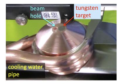
Figure 11.89: Target of SuperKEKB positron source
