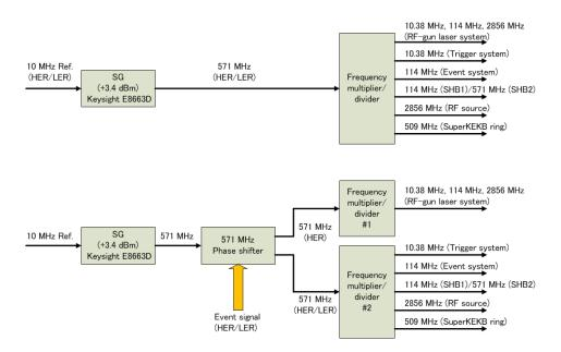
Figure 11.24: Configuration of the main drive system for the (a) KEKB injector linac, (b) SuperKEKB injector linac.
