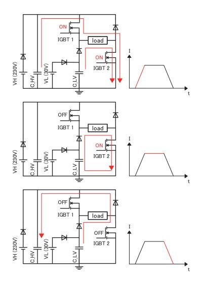
Figure 11.43: Conceptual circuit diagram of the pulse driver for quad magnet. Red allows shows the current path. Right side figures shows current profiles at corresponding states.
