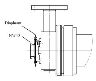
Figure 11.15: End part of the PF-type structures comprising of coupler, diaphragm and NW40 flange.
