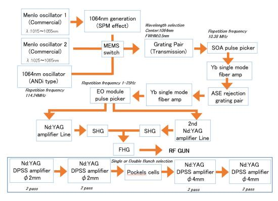
Figure 11.72: Layout of on the ground laser system.
