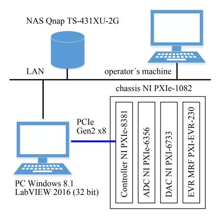
Figure 11.45: Components of the fast control system.
