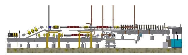
Figure 11.57: Layout of the thermionic gun, RF gun and the combination part at linac.
