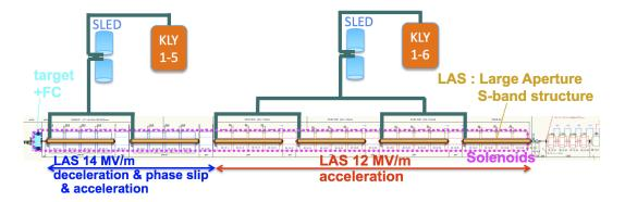
Figure 11.85: SuperKEKB positron capture section layout
