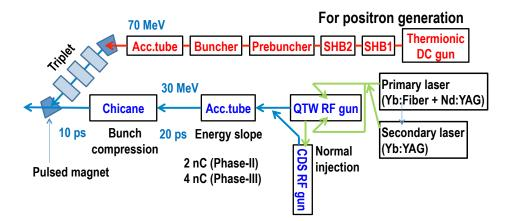
Figure 11.5: Layout of injector part.
