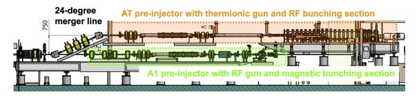
Figure 11.31: Double deck pre-injectors of SuperKEKB injector linac.
