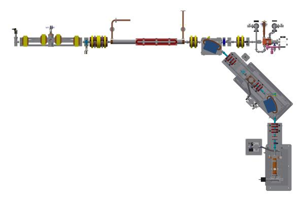
Figure 11.58: Layout of two RF guns at linac A1 unit.
