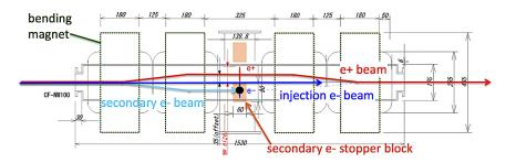
Figure 11.96: Beam separator and Secondary-electron stopper
