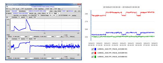
Figure 11.29: Display of waveform viewer (left) and archiver (right).
