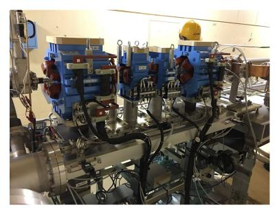
Figure 11.33: A set of pulsed quadrupole and steering magnets.
