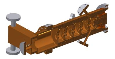
Figure 11.66: Configuration of CDS RF gun.
