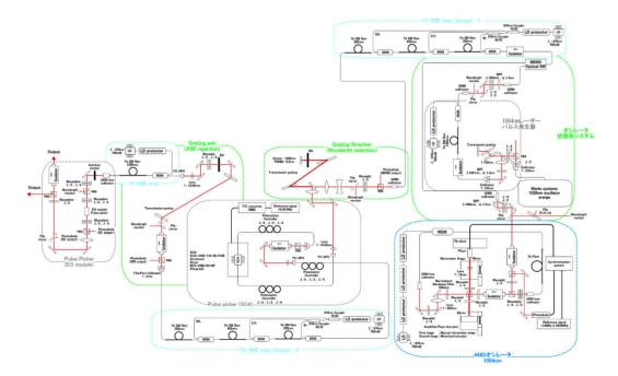
Figure 11.75: Fiber amplifier system.
