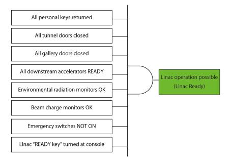
Figure 11.97: Safety conditions to be met before beam operation of the injector linac is allowed.
