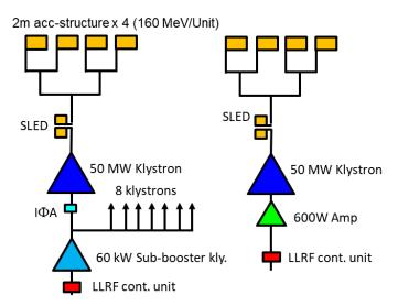
Figure 11.25: Klystron drive-line from a sub-booster klystron (left), and independent drive-line (right).
