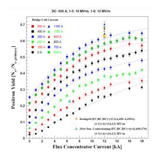
Figure 11.88: Positron Yield dependence on Capture section Parameters
