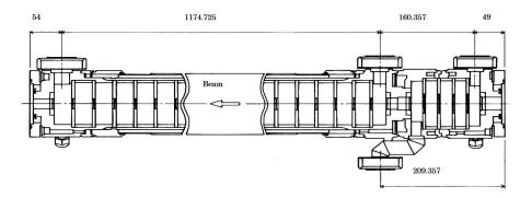
Figure 11.61: Configuration of prebuncher and buncher.
