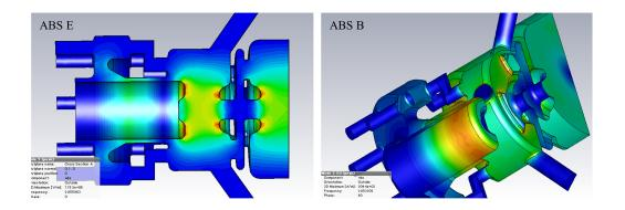
Figure 11.67: Distribution of the electric field and magnetic field near photocathode rod.
