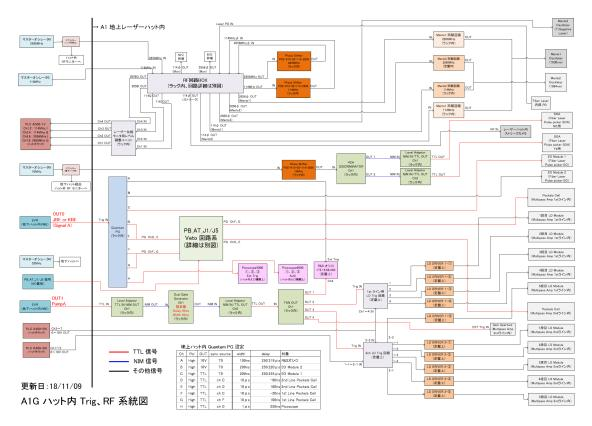
Figure 11.80: Layout of trigger system.
