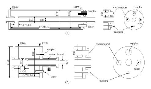
Figure 11.60: Configuration of SHB1 and SHB2.
