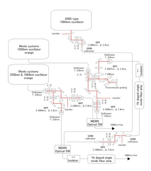
Figure 11.74: MEMS optics switch.
