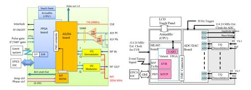
Figure 11.27: Block diagram of the LLRF control unit and RF monitor unit.
