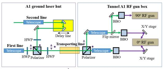
ullet Laser with vertical polarization,  $\clubsuit$  laser with horizontal polarization
