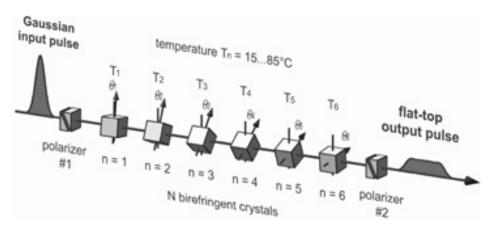
Figure 11.82: Pulse stacking technology.
