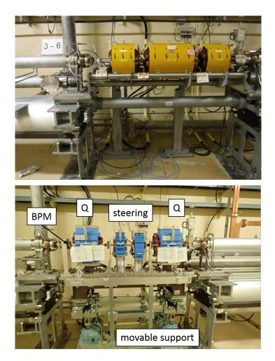
Figure 11.39: The upper photo shows old DC magnets before replacement. The lower photo shows newly installed unit.
