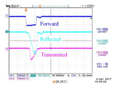
Figure 11.18: RF pulse shapes under vacuum breakdown at the first LAS structure in unit 15.
