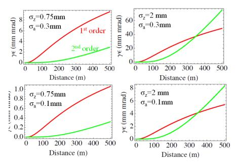
Figure 11.6: Analytical calculation of the projected emittance in several cases of the bunch length and the alignment error.
