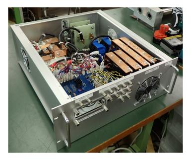
Figure 11.42: A photo of the pulse driver for quad magnet.
