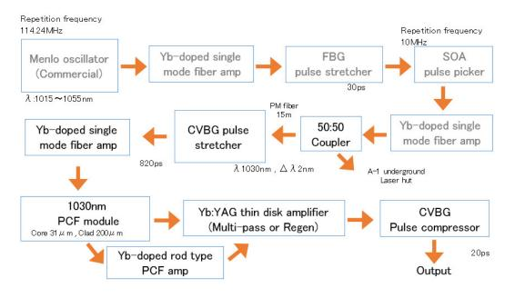
Figure 11.77: Layout of Underground laser system.
