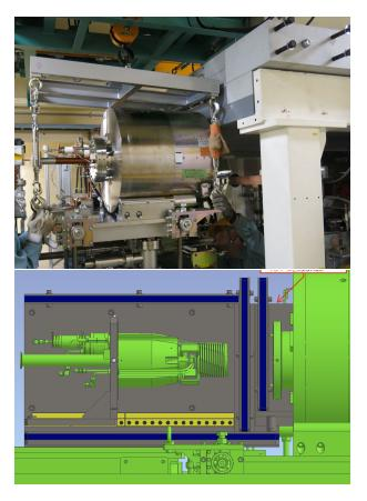
Figure 11.93: Quick exchange mechanism of FC and target
