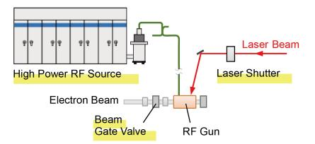
Figure 11.102: A sketch of RF source and laser beam used to generate beams with an RF gun.
