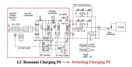
Figure 11.22: Simplified schematic diagram of the klystron modulator.
