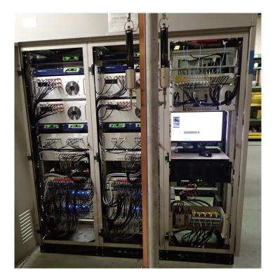
Figure 11.41: A photo of the standard unit for 4 quad and 4 steering magnets.
