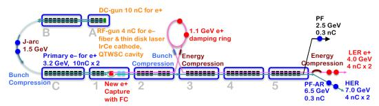
Figure 11.1: Overview of 600-m electron/positron injector linac with 60 accelerating units.
