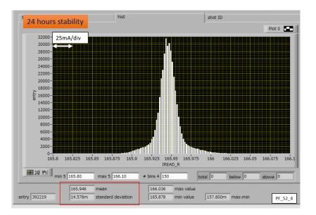
Figure 11.47: A histogram of the stability measurement of pulsed power supply for quad magnet.
