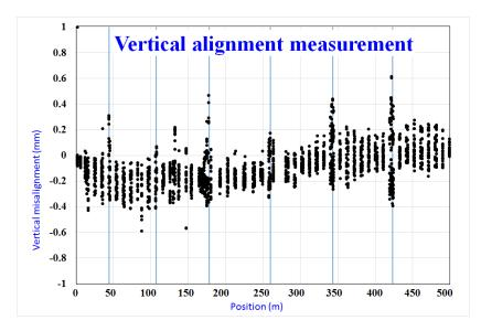
Figure 11.54: Ensemble of twenty data sets taken during two years, between May 2016 and June2018, measured by the laser QPD system.
