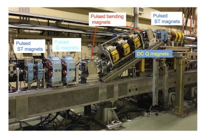
Figure 11.32: 24-degree beam merger line.
