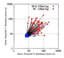
Figure 11.7: Initial offset to optimise the projected emittance.
