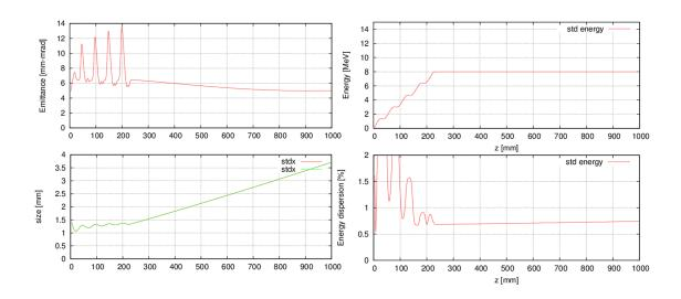
Figure 11.68: Beam tracking simulation result of emittance, beam energy, beam size and energy spread for 5 nC electron beam.
