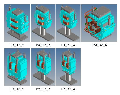
Figure 11.38: Appearance of installed pulsed magnets.
