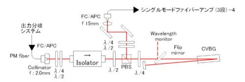
Figure 11.78: Layout of CVBG stretcher.
