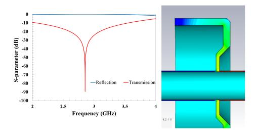
Figure 11.71: RF shielding simulation result for electron beam heating type photocathode plug choke structure.
