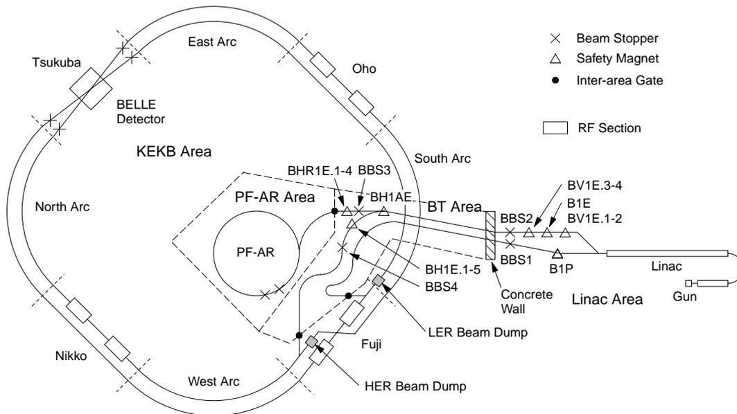
Fig. 9. Access control areas and devices for access safety.
