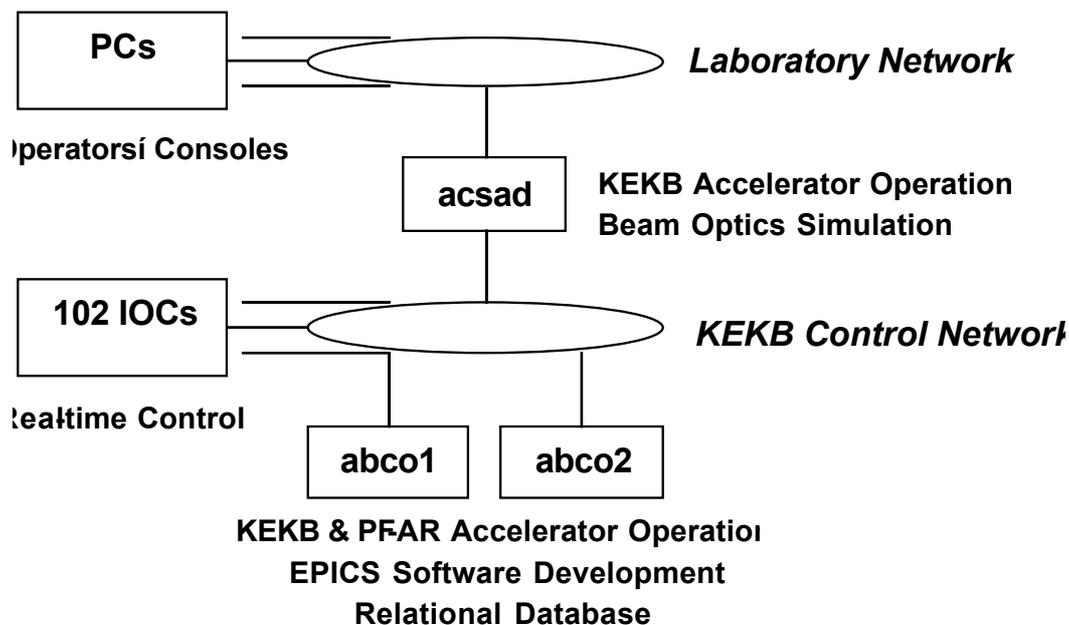
Fig. 4. New System Configuration of Server Workstations
