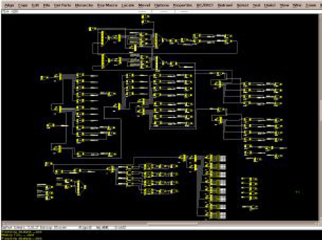
Fig. 6. An example EPICS database as CAPFAST schematic
