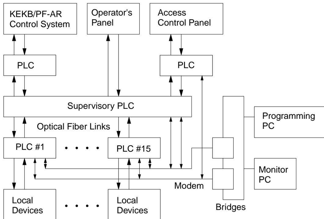
Fig. 10. Architecture of the radiation safety system.
