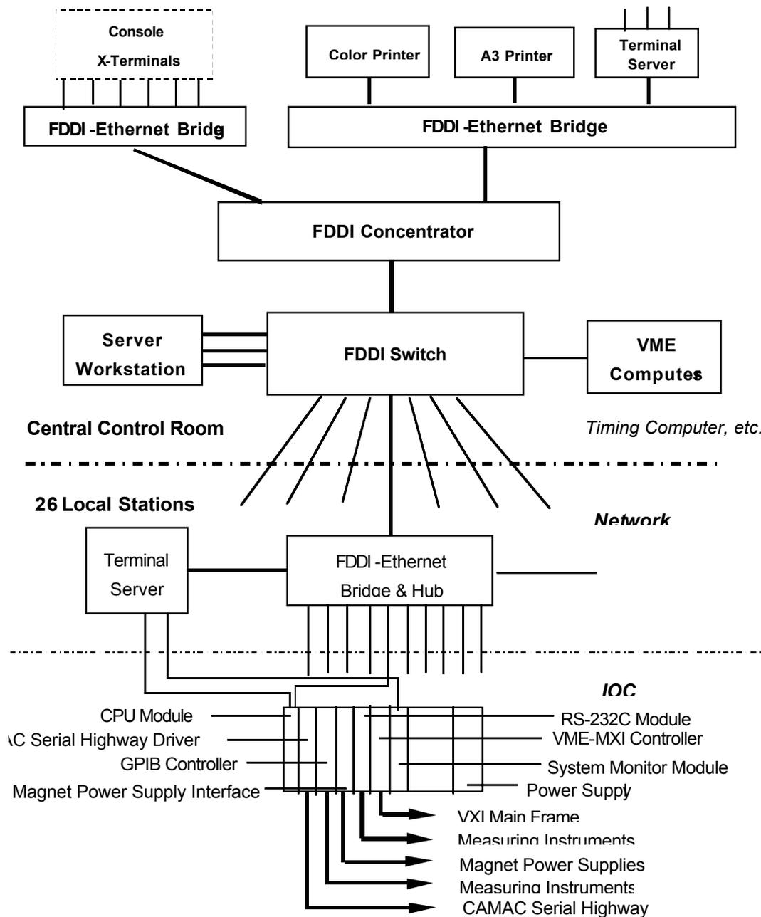
Fig. 5. Schematic configuration of the KEKB accelerator Control Computer system
