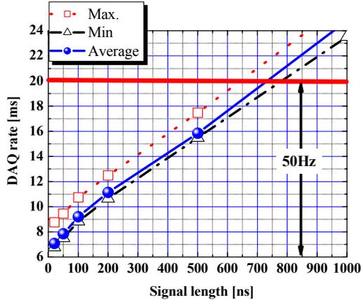
Fig. 2: Result of data acquisition speed. Square (red), triangle (black) and circle (blue) mean maximum, minimum and average data acquisition time.
