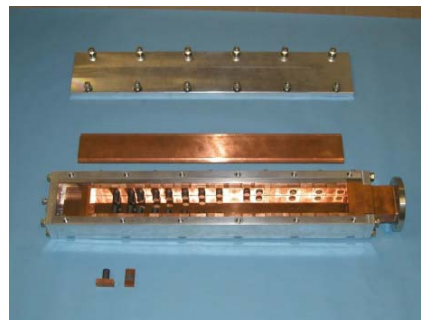
Figure 14: Photograph of the dummy load.
