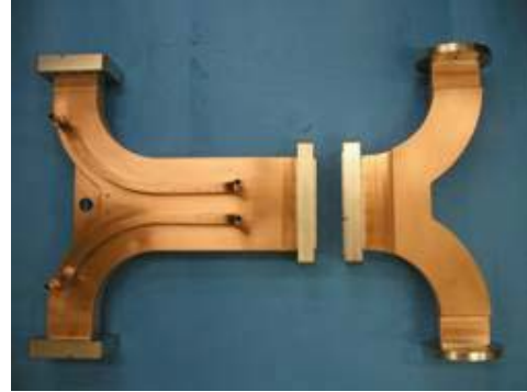
Figure 8: Whole view of 3dB-hybrid coupler (left) and waveguide for low power RF measurement (right).
