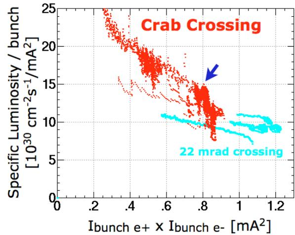
Figure 7: Specific luminosity per bunch with crab crossing (red) comparing to crossing angle (blue) as a function of the product of bunch current. The highest  $\xi_y \sim 0.088$  was achieved at the arrow.
