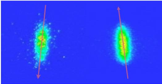
Figure 6: Images taken by streak cameras, which locate as Fig. 2, show tilt of the bunches in the LER (left) and the HER (right)[11].
