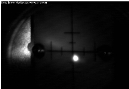
Figure 3: Transverse beam profile captured by video encoder system in the KEK injector linac.
