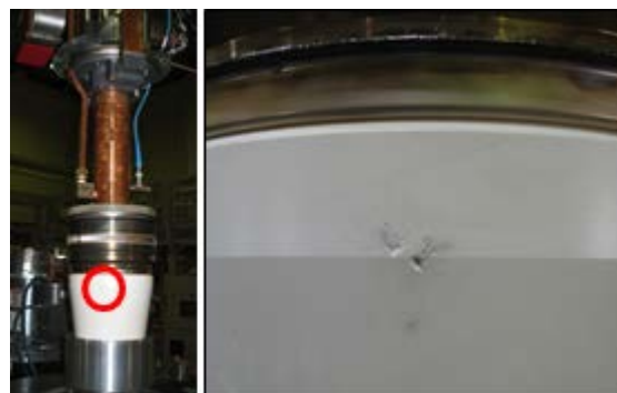
Figure 4: The insulator damage at a klystron and observed penetration hole at the ceramic insulator.
