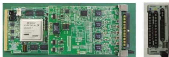
Figure 1: The FPGA control board.
