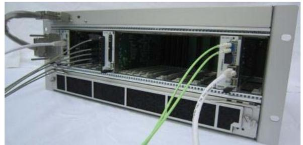
Figure 7: FPGA Control Board and Arithmetic Processing Board for BPM system.
