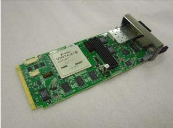
Figure 4: The Arithmetic Processing Board.
