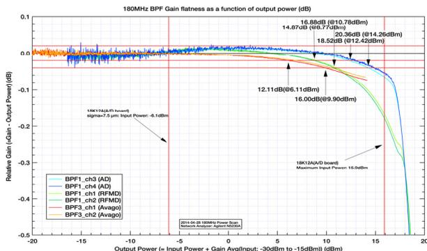
Figure 4: Amplifier linearity curve in the BPF circuitry is shown. AD (Blue) shows wide linearity, Avago (Red) shows moderate characteristics and RFMD (Yellow) shows narrow linearity.
