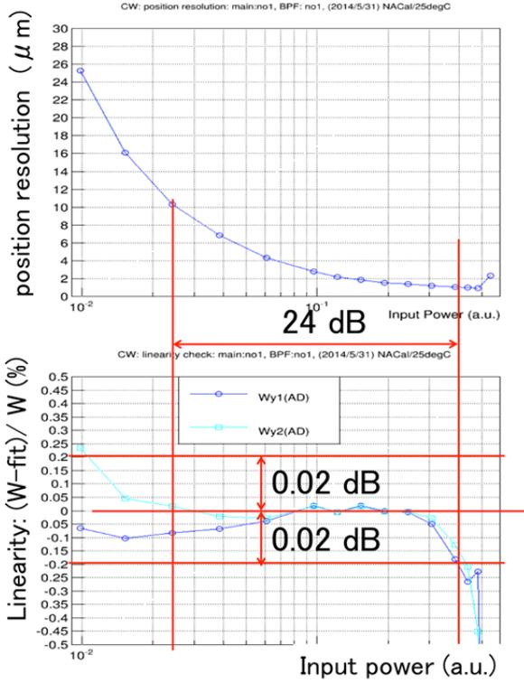
Figure 6: Upper plot shows BPM readout system resolution at ideal condition. Lower plot shows system linearity: we have 24 dB with  $\pm 0.02$  dB linearity range.
