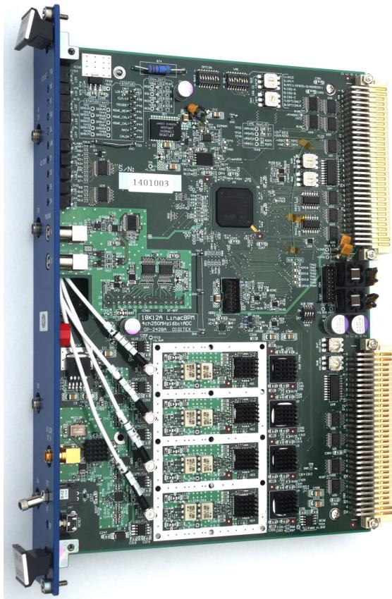
Figure 2: An photograph of prototype of BPM readout board (called 18K12A) is shown. This is a double width module. A BPF board is attached on bottom of a main (ADC) board. The output from BPF board is fed to the main board via four coaxial cables.
