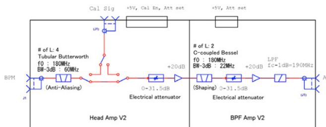
Figure 3: Block diagram of Band Pass Filter board (one channel is shown). It equips calibration pulse input selector. First Butterworth filter (60 MHz) cut tails that exceed ADC's Nyquist window (125 MHz – 250 MHz) and second Bessel filter (22 MHz) forms total bandwidth and burst length (60 ns). Each stage has an electrical attenuator and an amplifier to set an adequate level.
