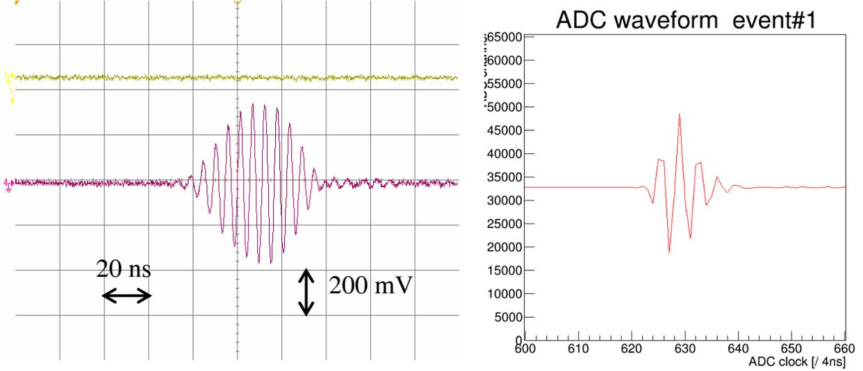
Figure 5: (a) BPF output waveform and (b) ADC sampled data points (2nd Nyquist zone under sampling).
