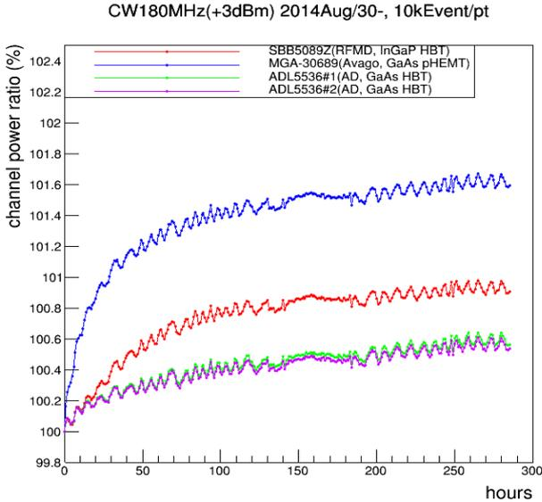
Figure 7: Amplifier gain drift is shown. Vertical axis is normalized channel power and horizontal axis is elapsed time. DUTs were tested in a thermostatic chamber.
