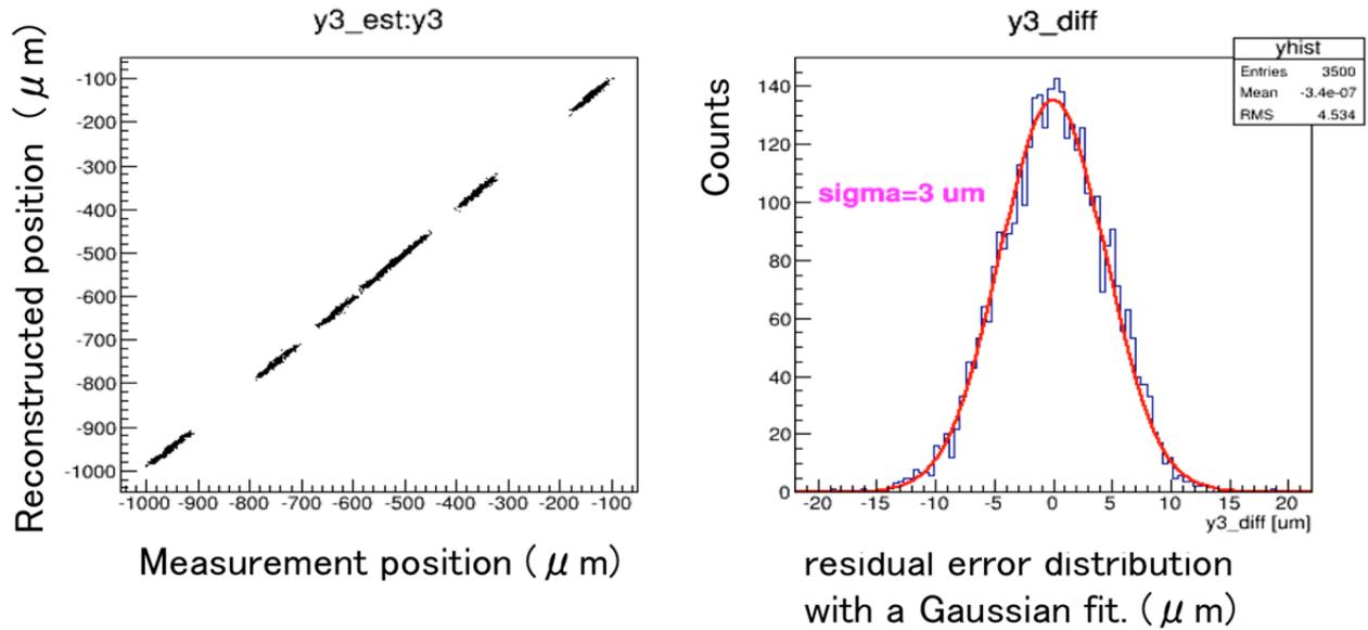
Figure 8: Left plot shows reconstructed position vs. measured position. Right plot shows residual error distribution histogram.
