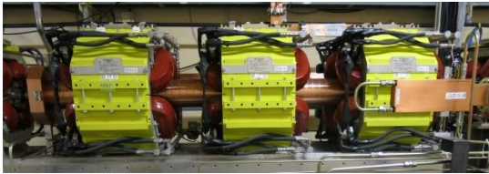
Figure 6: Densely placed quadrupole magnets for transportation of large emittance positrons. They are overlapping with the accelerating structures.
