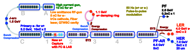
Figure 1: Layout of injector linac and its beam delivery to multiple experimental facilities.
