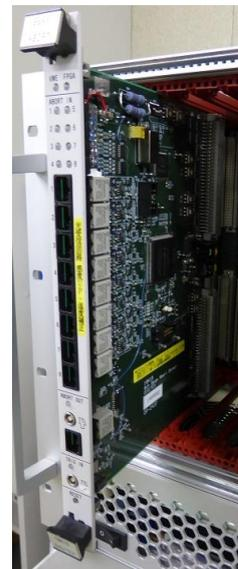
Figure 2: Picture of the VME-based 8ch beam abort optical input module (18K15).
