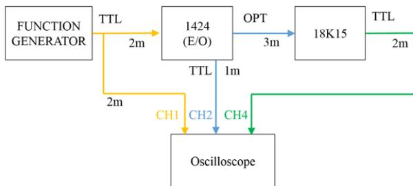
Figure 5: Schematic diagram of the response time measurement.
