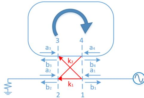
Figure 2: Schematic diagram of the resonant ring.
