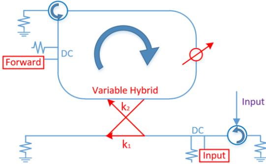
Figure 3: Structure diagram of the resonant ring.
