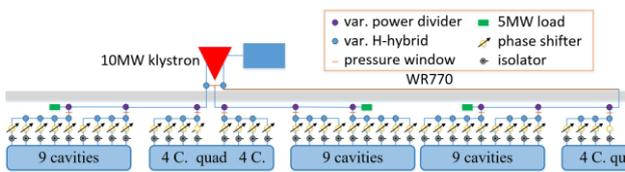
Figure 1: Power distribution system for ILC.
