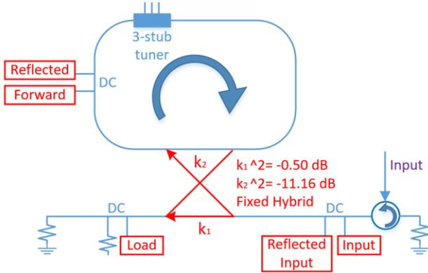
Figure 7: Resonant ring with 3-stub tuner.
