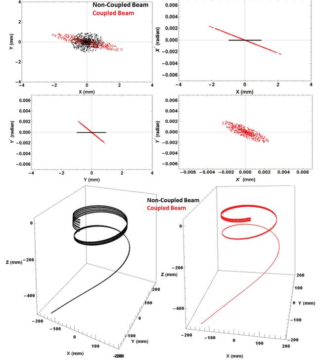
Figure 3: The above four plots are the required phase space at the matching point ( $Z = -500$  mm). The black points show the beam phase space without coupling and red points show with coupling. Bottom two plots are showing the beam injection with and without coupled beam.
