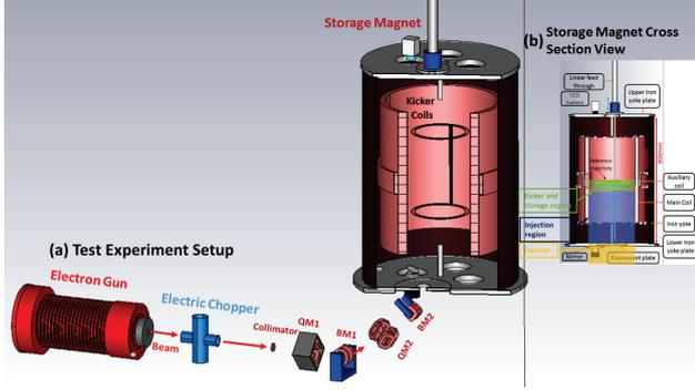
Figure 2: (a) A diagram showing the 3D schematic of spiral injection test experiment. (b) The schematic of the storage magnet with monitors and reference trajectory.
