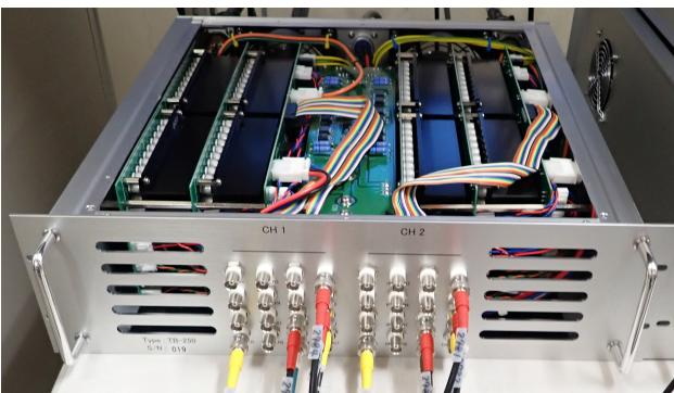
Figure 3: Type TB-250 Bipolar power supply for pulsed steering magnet.
