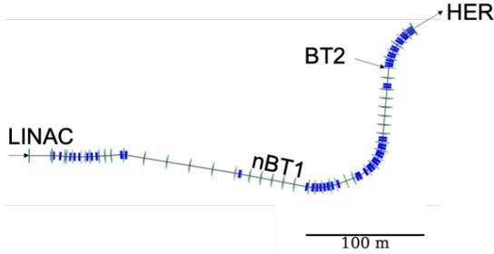
Figure 7: New straight beam transport line with two achromatic segments of nBT1 and BT2.
