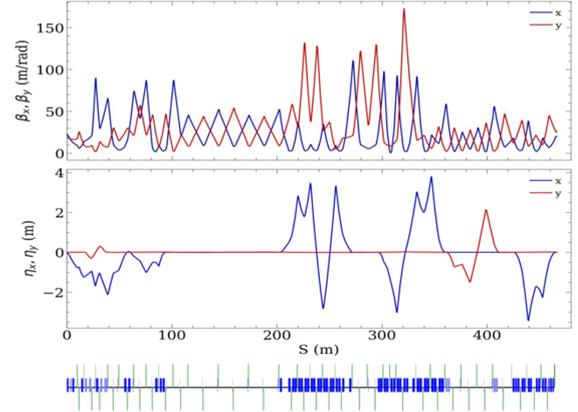
Figure 2: Nominal 7-GeV electron beam transport optics with dispersion functions shown in blue and red for the horizontal and vertical directions, respectively.
