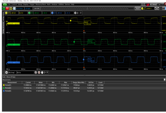
Figure 7: Period jitter measurement from three EVR outputs.
