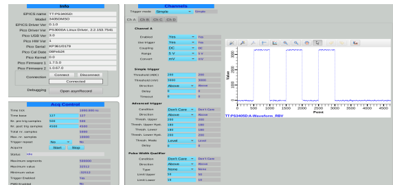
Figure 4: The PicoScope captures a waveform from EVR which triggers from sequence of events.
