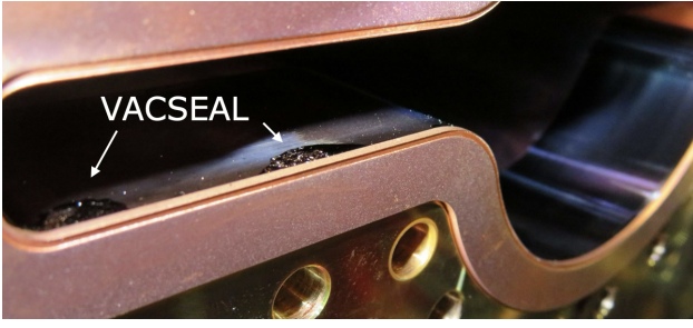
Figure 6: VACSEAL as black stains in the MO-type flange connection.
