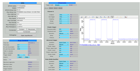
Figure 5: The GUI panel shows Picoscope captures the output pulse from an EVR.
