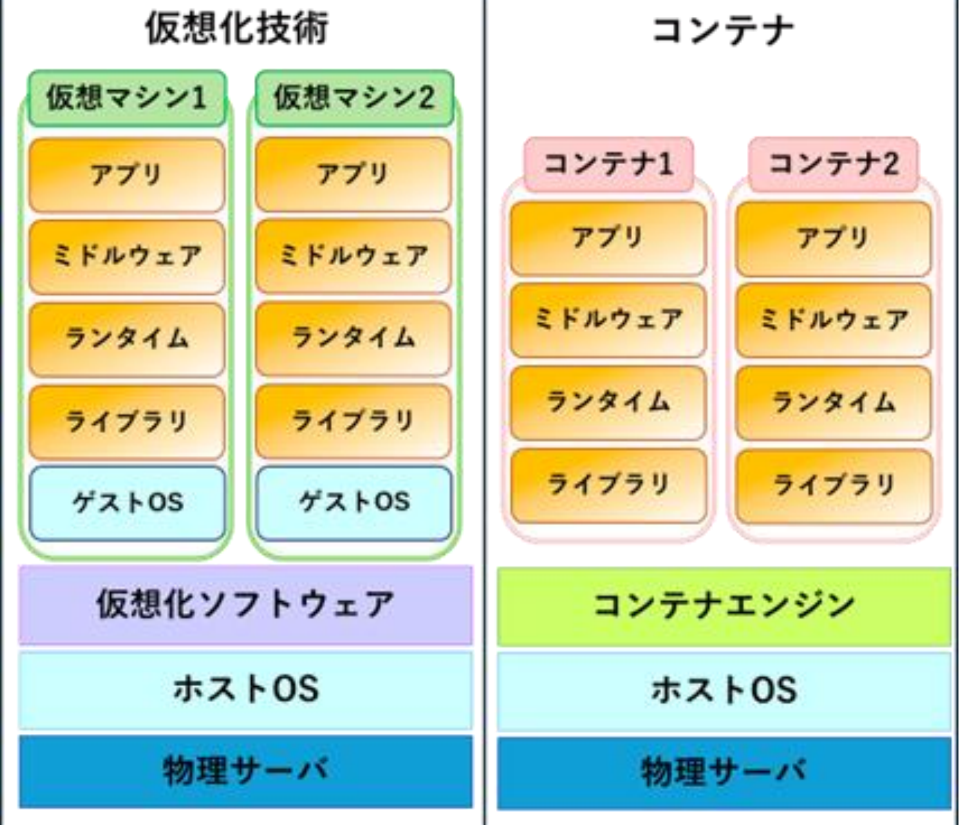
Figure 6: Layered architecture comparison of virtual machine and container.
