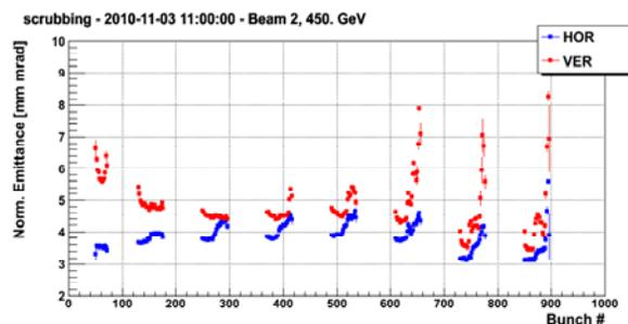
Figure 6: Bunch by bunch emittance showing the blow-up of some bunches due to electron cloud instabilities.
