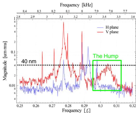
Figure 2: Typical tune spectrum resulting from residual beam oscillations. Also visible is the unknown perturbation source known as “the hump”.
