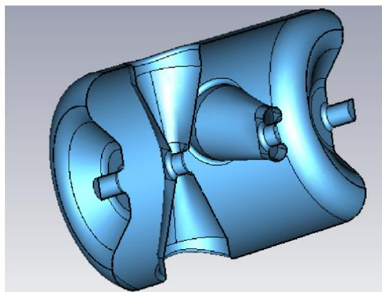
Figure 2: Double spoke resonator cavity, with an accelerating gradient of 8 MV/m and a geometric  $\beta$  of 0.57.
