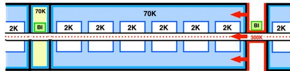
Figure 5: Interconnects between hybrid cryomodules may be either warm or cold ( $\sim 70$  K).
