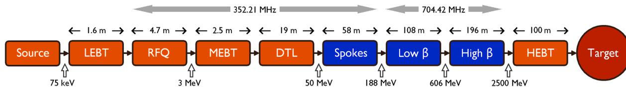
Figure 1: The “2011 hybrid” baseline layout of the ESS linac. Red sections – the RFQ, the DTL, and the Low-, Medium- and High- Energy Beam Transports, (LEBT, MEBT, and HEBT) – are normal conducting. Blue sections – spoke resonators, low- $\beta$ , and high- $\beta$  elliptical cavities – are superconducting.
