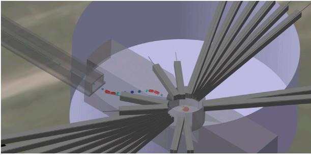
Figure 4: Interface between the HEBT, the rotating tungsten disk target, moderators, and the 22 neutron beamlines.
