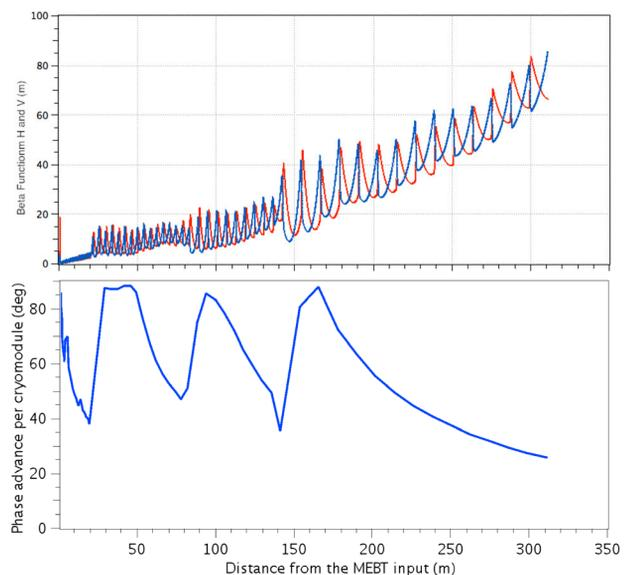
Figure 6: Transverse beta functions (top) and the longitudinal phase advance per cryomodule (bottom), for most of the ESS linac.
