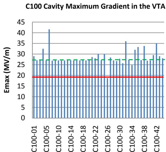
Figure 4: A summary of the C100 cavity testing performance as measured in the VTA. The dashed line shows the administrative limit of 27 MV/m, while the red line shows the design specification of 19.2 MV/m.
