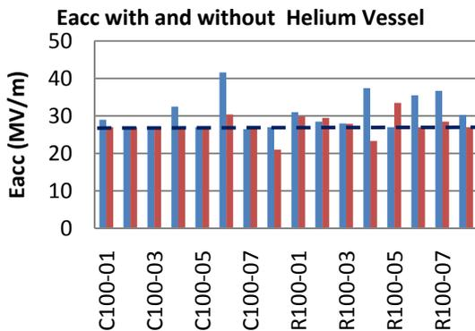
Figure 2: A comparison of 16 cavities' RF performance before (blue) and after (red) helium vessel welding. The administrative limit of 27 MV/m is shown by the dashed line. Note, the maximum gradient possible in a helium vessel is ~34 MV/m.
