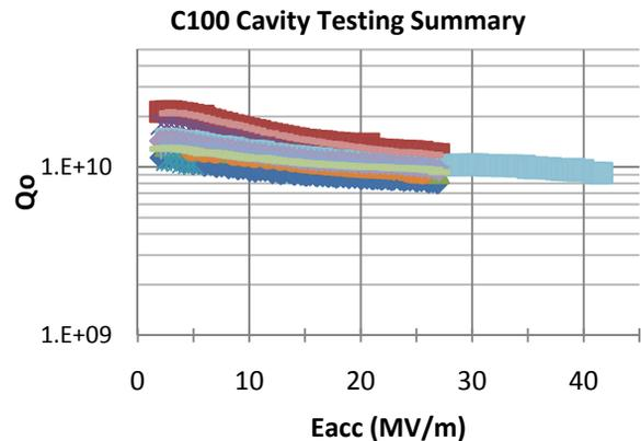
Figure 5: A sample of 12 C100 cavities RF performance demonstrating the excellent cavities that are being produced using the 12 GeV cavity processing cycle.
