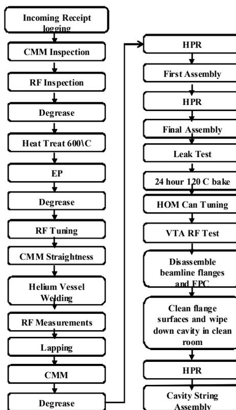
Figure 1: This is the process flow chart that is being followed for the C100 cavity production process for the 12 GeV upgrade.
