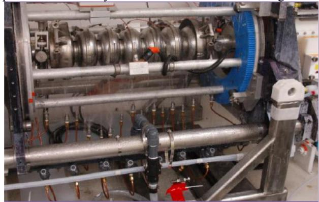
Figure 3: A 12 GeV upgrade cavity in the electropolishing tool. The spray cooling nozzles are shown at the bottom, and maintain the cavity at 20°C.
