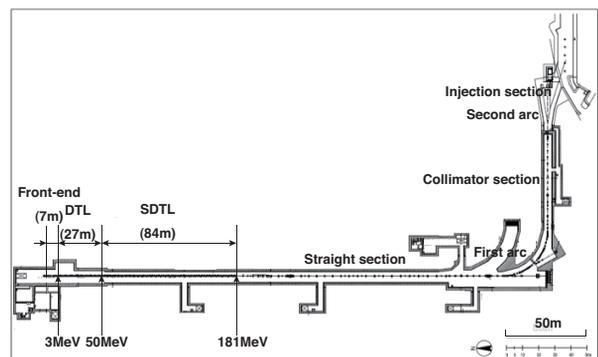
Figure 1: Scaled layout of J-PARC linac.
