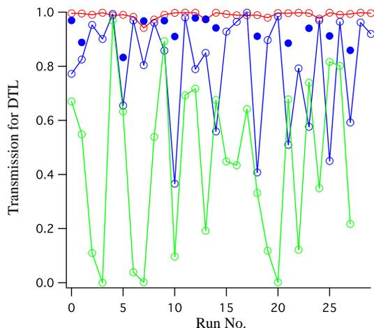
Figure 4: The simulated transmission efficiency. Red, blue, and green open circles, respectively, denote the results with the DTQ alignment error of  $\pm 0.1$  mm,  $\pm 0.2$  mm, and  $\pm 0.3$  mm. The blue filled circles show improvement of the transmission efficiency by beam steering for some cases with  $\pm 0.2$  mm DTQ misalignment.
