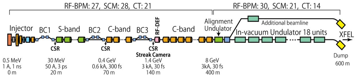
Figure 1: SACLA accelerator layout and the number of beam monitors.
