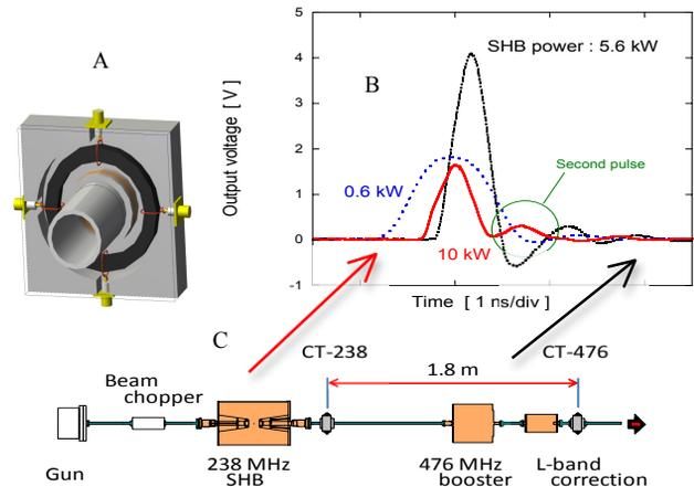
Figure 5: A, DCT. B, Bunching of an electron beam observed with the DCT, when changing the SHB rf power. C, Injector layout.
