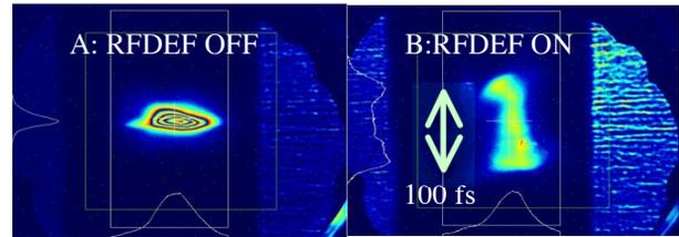
Figure 4: A, the beam profile taken with the Ce:YAG screen and B, the beam image pitched by the RFDEF.
