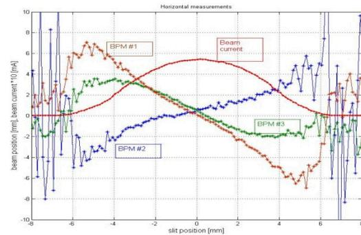
Figure 5: The measured dependence of the beamlet position vs. the slit position at three BPMs and the beam current through the slit.
