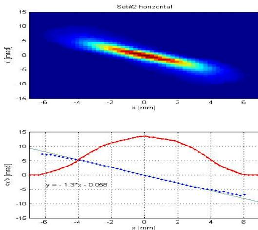
Figure 4: The measured horizontal emittance in the SNS MEBT (top). Beam current through the slit (bottom, red), and  $\langle x' \rangle$  (bottom, blue) vs. slit position.
