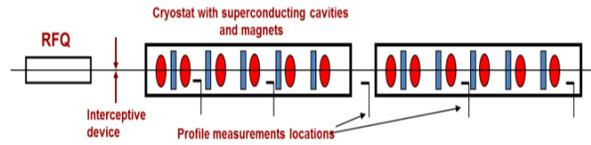
Figure 1: A layout of the measurement arrangement.
