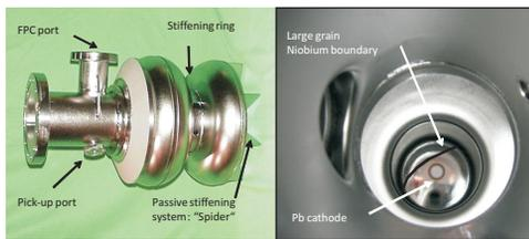
Figure 1: The picture on the left shows the 1.6 cell SC gun cavity after production and assembly of all ancillary components at JLab, the right picture shows the greyish lead cathode on the half cell backwall. The cavity is equipped with the TTF-III power coupler.
