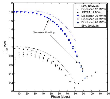
Figure 6: Measured beam kinetic energies for 12 and 20 MV/m launch field versus phase compared to ASTRA and longitudinal tracking simulations.
