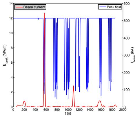
Figure 5:  $E_{peak}$  and average beam current versus time during the observation of cavity field trips at specific cathode positions. Sometimes currents above 500 nA were observed.
