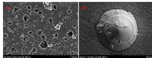
Figure 4: The pictures show SEM images (taken at FHI) of arc deposited lead samples by A. Soltan Institute similar to the gun cavity cathode. Small surface defects, droplets and tip on tip like structures in the 1-20  $\mu\text{m}$  scale were observed.
