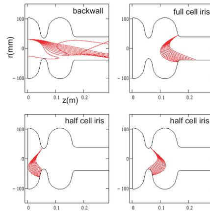
Figure 3: Tracking studies of possible dark current sources by V. Volkov for the 1.6 cell gun cavity.
