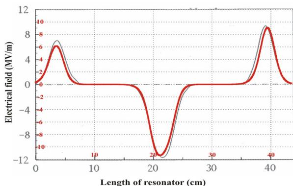
Figure 5: Measured (black) and calculated with DYNAMION (red) longitudinal electrical field on the axis along the 108 MHz GSI-LIGHT-buncher.
