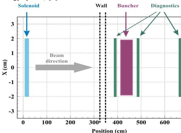
Figure 3: Scheme of the LIGHT beam line
