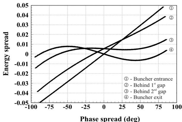
Figure 6: Bunch rotation with the 3-gap buncher. Input energy spread  $\pm 5\%$ , input divergence  $\pm 43$  mrad.
