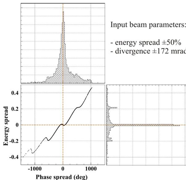
Figure 7: A longitudinal beam phase portrait at the end of the transport line.
