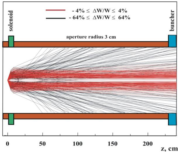
Figure 2: Typical particle trajectories along the beam line. Red lines show particle with input energy spread of  $\pm 4\%$ .
