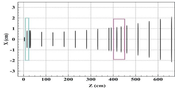
Figure 4: Beam envelopes of the monoenergetic beam with small initial transverse divergence of  $\pm 43$  mrad along the recent transport line with solenoid (blue box) and buncher (magenta box).
