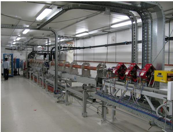
Figure 2: Linac and RF waveguide distribution inside the linac tunnel. The waveguides are hung from the roof and couple to the accelerating structures from above.
