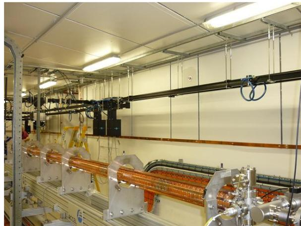
Figure 3: Linac and RF distribution after waveguide modification. The new power splitter and phase shifter can be seen just left of the centre of this image. The additional waveguide can be seen extending left, below the original piece.
