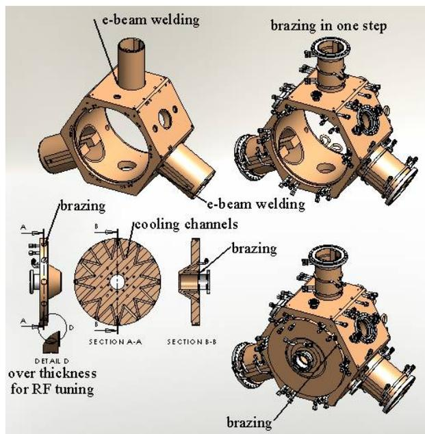
Figure 2: Main assembly steps of initial specified design.
