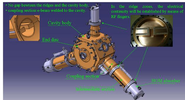
Figure 1: General design of the copper prototype.
