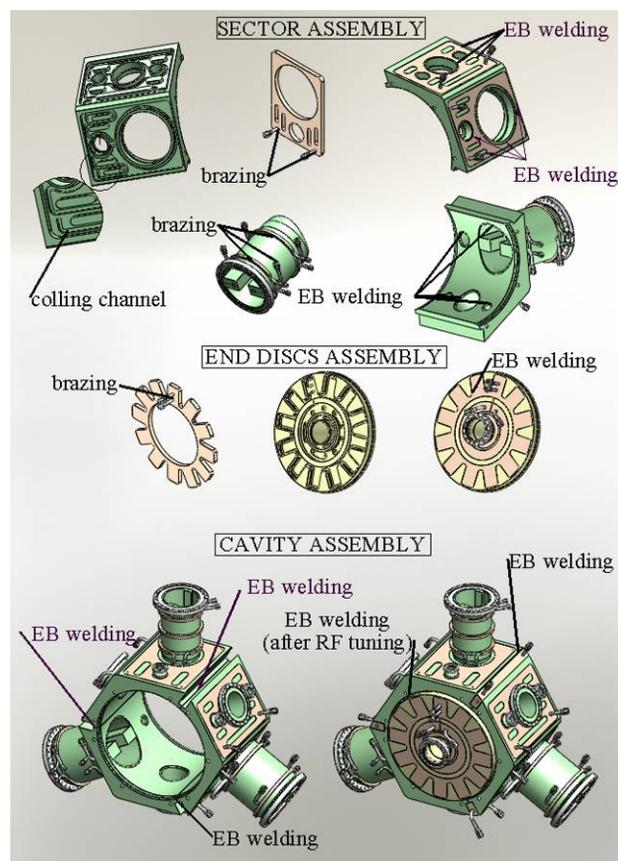
Figure 4: Main assembly steps of alternative design.
