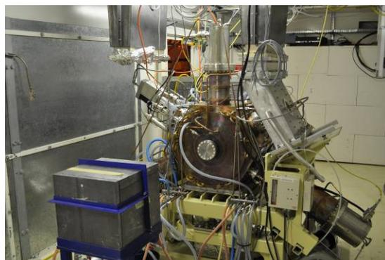
Figure 6: RI cavity in the RF power teststand.
