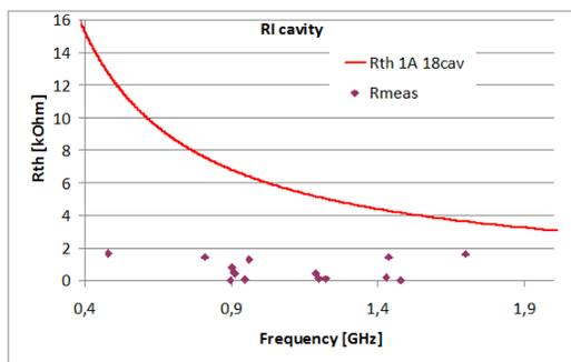
Figure 5: RI cavity - longitudinal HOM measurements.
