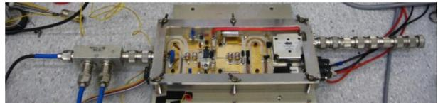
Figure 1: ELTA/SOLEIL 650 W RF module under test.
