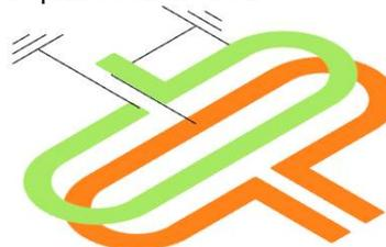
Figure 9: Printed balun transformer.
