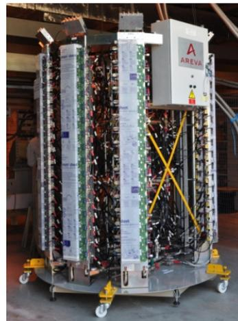
Figure 2: First 75 kW amplifier tower combining 128 RF modules.
