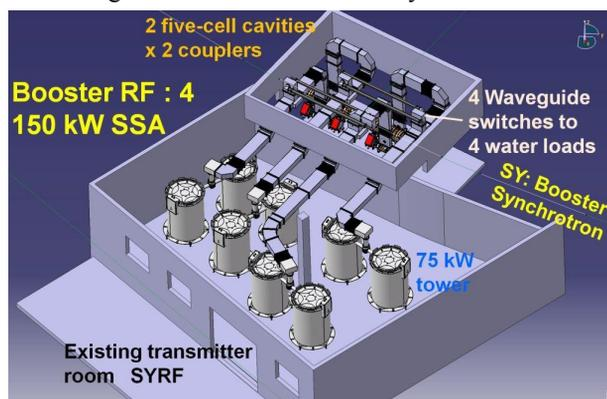
Figure 5: Four SSA replacing the klystron on the booster.
