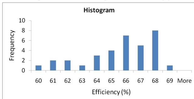
Figure 4: Distribution of measured efficiency for 34 RF modules after 1000 h run test.
