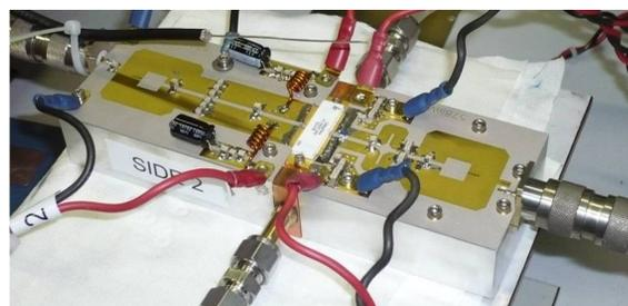
Figure 10: RF module using printed balun transformers.
