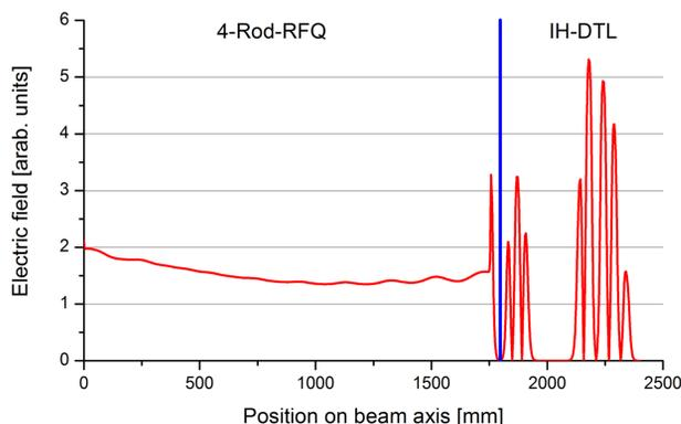
Figure 4: Field distribution on the beam axis along RFQ-IH-DTL combination. The blue line separates the both cavities. The voltage ratio must be 26 so that both accelerators have a strong field distribution and no cavity is suppressed. In this case the RFQ has no flatness of the RFQ field distribution.
