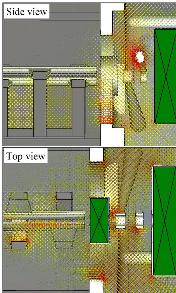
Figure 3: Side and top view on the coupling area. The RFQ is on the left and the IH-DTL is on the right side. The beam goes to the right direction. The arrows represent the magnetic fields and thus the inductive coupling. The inductive coupling connects the RFQ with IH-DTL.
