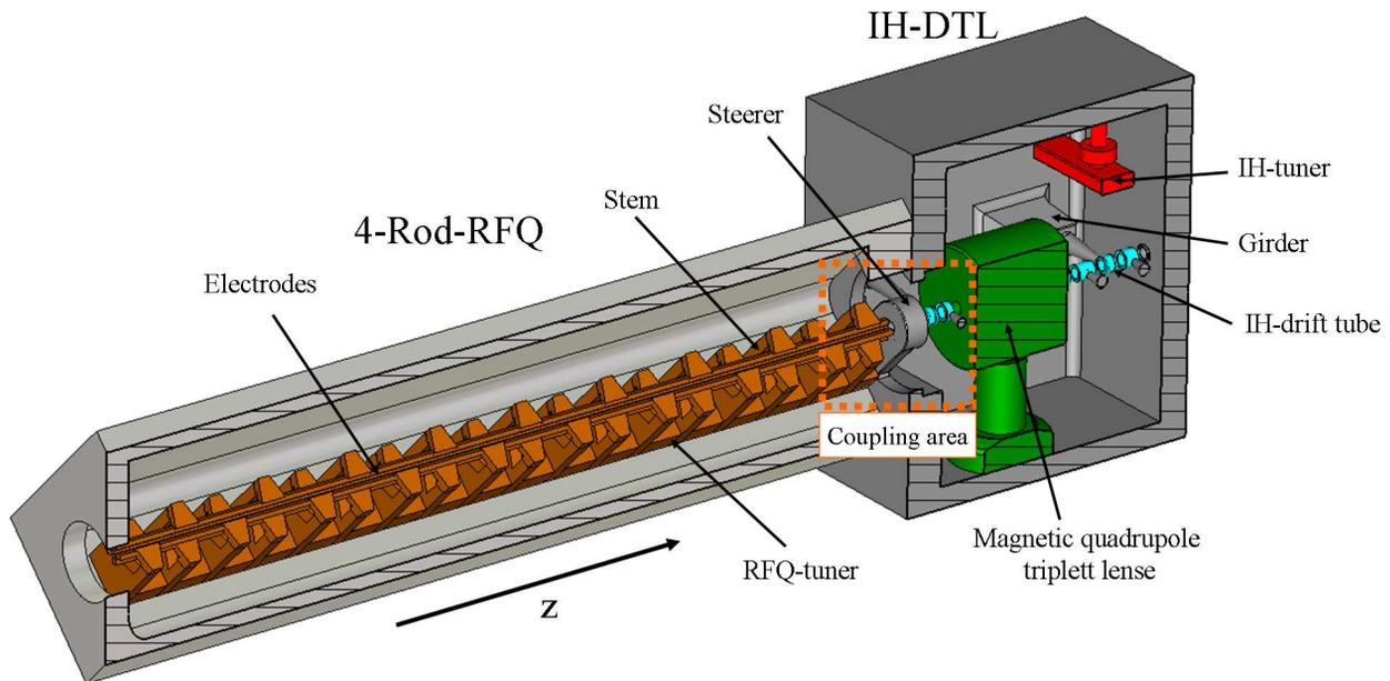
Figure 2: Cross sectional view of the coupled RFQ-IH-DTL combination for FRANZ. The 4-Rod-RFQ is shown left and the IH-DTL on the right side. In coppery are the RFQ-electrodes and stems, in the coupling area is in the gray the xy-steerer. The drift tubes are colored in cyan and the magnetic quadrupole triplet lens is shown in green. In the IH-DTL is represented in red the dynamic tuner.
