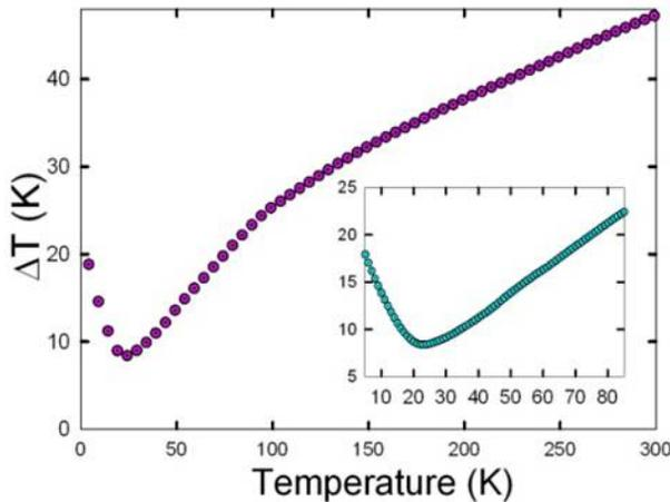
Figure 2: Surface temperature rise after 1 ms RF pulse as a function of initial gun temperature (Gradient 60 MV/m).
