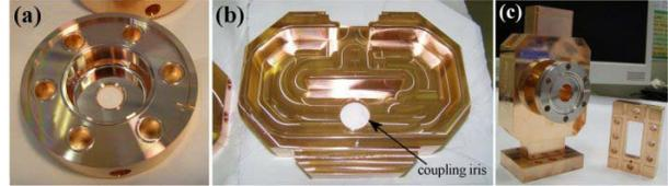
Fig. 3: (a) single cell; (b) input and (c) output couplers.
