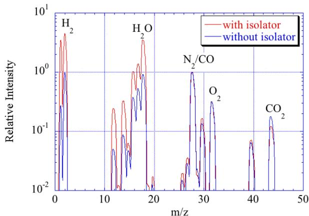
Figure 8: Residual gas spectrum with/without isolator (relative intensity was normalized for  $N_2/CO$ ).
