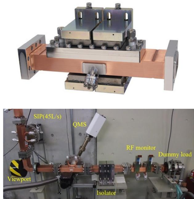
Figure 4: Prototype vacuum isolator (above: a viewport is located to observe ferrite surface) and setup for a high power test (below).
