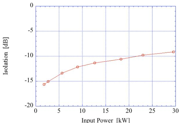
Figure 6: Isolation of prototype isolator as a function of input power.
