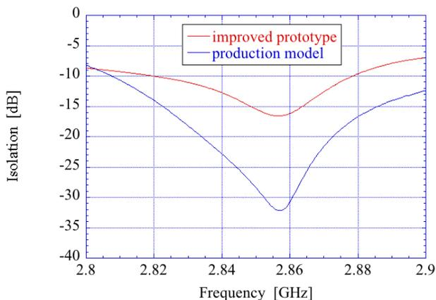
Figure 7: Improvement of isolation by expanding ferrite and external magnets.
