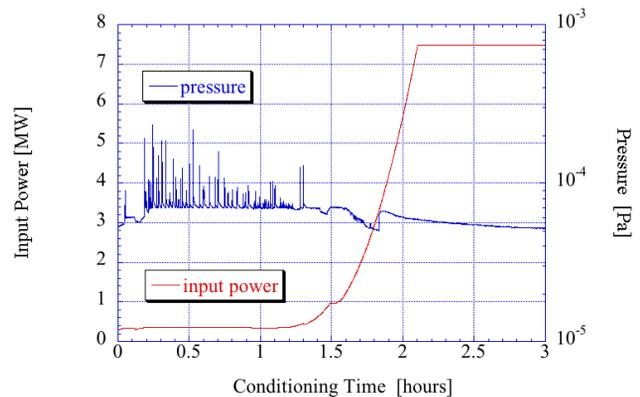
Figure 5: Input power and vacuum pressure history of RF conditioning of prototype isolator (normal direction).
