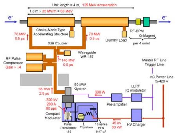
Figure 2: Configuration of C-band accelerator system.
