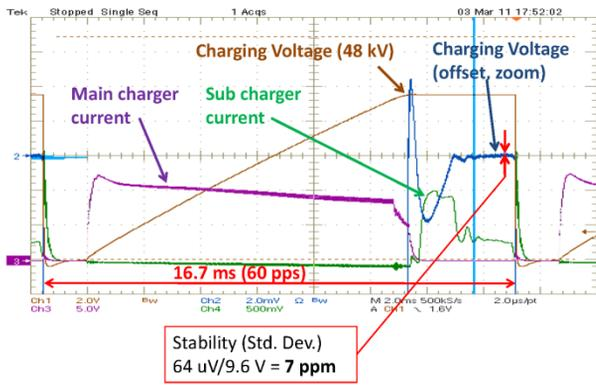
Figure 3: Typical waveform of the PFN voltage and the charging current. The blue waveform shows the waveform of the PFN voltage around the target voltage.
