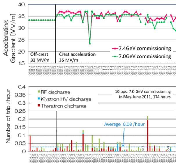
Figure 5: (Upper) Accelerating gradient of each RF unit, in typical operational. (Lower) Trip rate of each RF unit.
