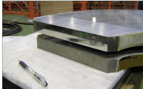
Figure 1: Picture of core cutting surfaces. The lower cutting surface is obtained after water jet cutting and the upper one is after polishing with diamond powder.
