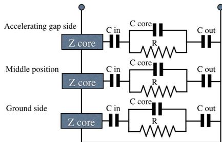
Figure 8: A circuit diagram of the water tank that stacks three MA cores.  $C_{in}$  and  $C_{out}$  represent the capacitances of the inner and outer space between water tank and cores, respectively.  $C_{core}$  represents the capacitance in radial direction of core and is a sum of the capacitances between ribbon layers.  $R$  represents the resistance due to the rust on the core cutting surface.
