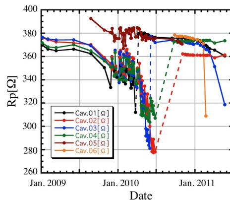
Figure 2: The results of impedance measurements of MR RF cavities. The horizontal axis shows the date and the vertical axis shows the real part of the cavity impedance at the resonance frequency. The broken lines represent the core replacements.
