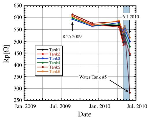
Figure 4: The results of impedance measurements of RF cavity #3 each water tank.
