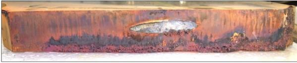
Figure 7: Picture of cutting surface of the core at the accelerating gap side in water tank #5 that showed large impedance reduction. The cutting face edge was damaged due to the RF voltage.
