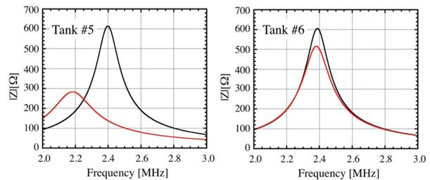
Figure 5: Impedance curve of water tanks #5 and #6. The horizontal axis shows frequency and the vertical axis shows absolute value of tank impedance. The black and red line represents the impedance data at Aug. 25, 2009 and Jun. 1, 2010, respectively.
