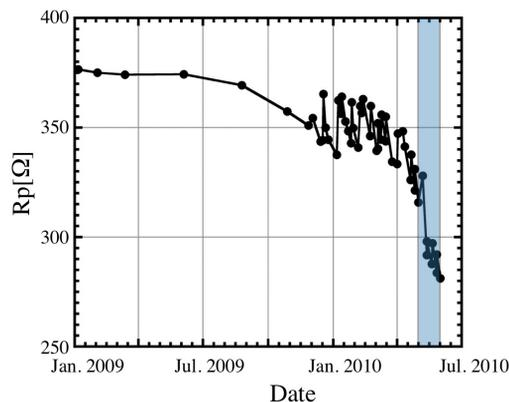
Figure 3: The results of impedance measurements of RF cavity #3. The blue region represents May 2010.
