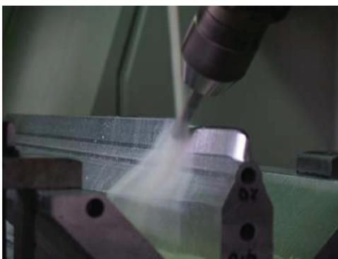
Figure 4: Vane-tip machining of an aluminum test segment with the ball-end mill.
