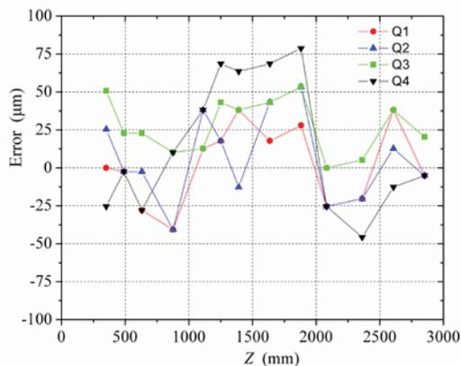
Figure 7: Measurement result of the vane-tip gaps at the position of the tuners and vacuum ports.
