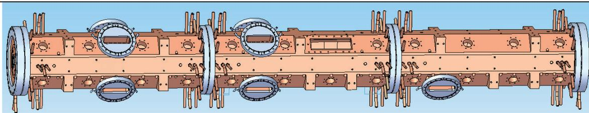
Figure 3: 3D model of the CPHS RFQ.
