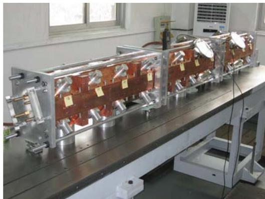
Figure 8: Assembled CPHS RFQ for the pre-braze tuning.
