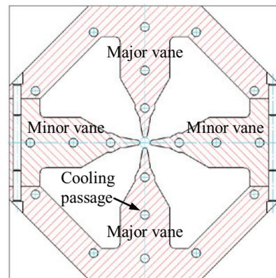
Figure 1: Cross section of the first segment at a fixed longitudinal position.
