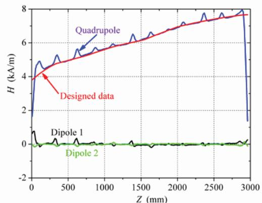
Figure 10: Field distribution of the quadrupole and dipole modes after the pre-braze tuning.
