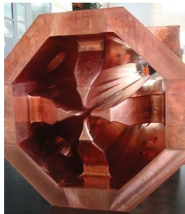
Figure 6: Assembled first segment of the CPHS RFQ.
