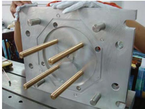
Figure 9: The dipole stabilizer rods.
