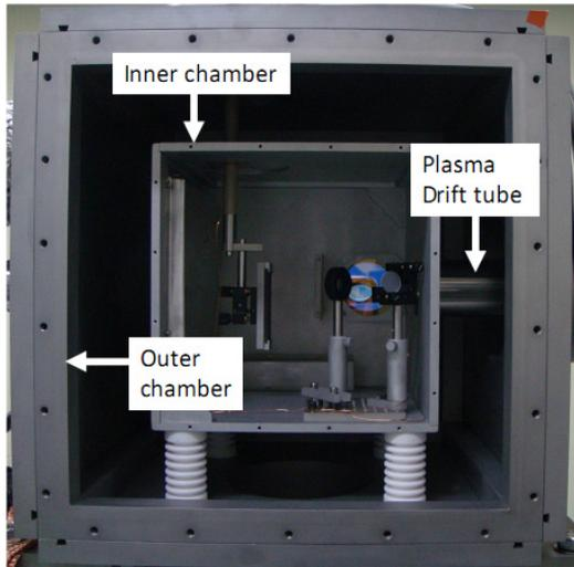
Figure 1: LIS target chamber at IMP
