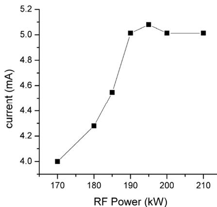
Figure 9: Beam current from RFQ vs. RF power of RFQ
