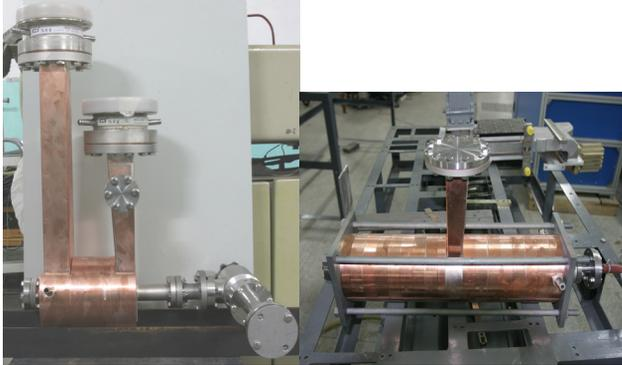
Figure 3: The welding rf gun and 9Cell accelerating tube
